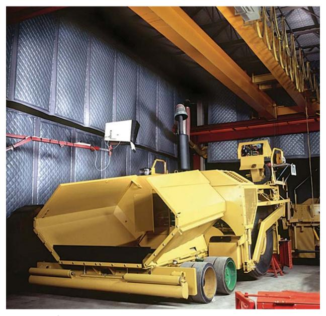
Durable, SONEX® Curtain BB is a composite that features sound-absorptive WILLTEC™ foam quilted with a vinyl facing on one side and bonded to a reinforced noise barrier material. This product provides excellent sound transmission loss and sound absorption performance. SONEX Curtain BB is ideal for use as barriers, independent walls, partitions or acoustical screens to isolate noisy machines or specific areas.
